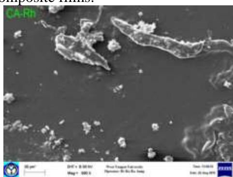
Figure 5. SEM micrograph of cellulose acetate-rice husk (CA- RH 4) composite film
